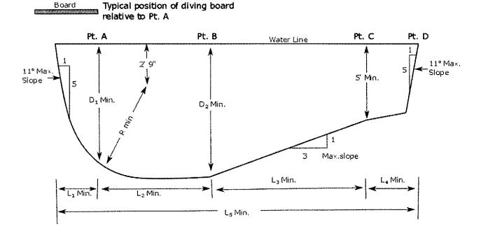
Note: L<sub>4</sub> is a minimum dimension to allow sufficient length opposite the board. This may of course be lengthened to form the shallow portion of the pool.
